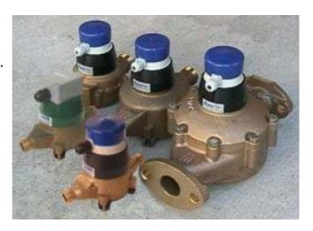
The MES20, MES25, MES32 and MES4050 nutating disc magnetically coupled positive displacement pulse output flowmeters are suitable for a wide range of precision batching and flowrate monitoring applications, operating from low to high flow ranges.
